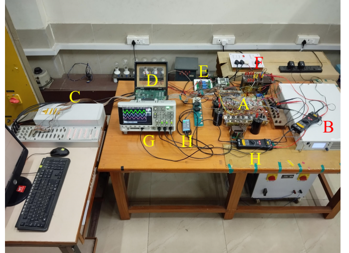
Fig. 20. Hardware-based experimental setup showing A: proposed MLI, B: power supply, C: dSPACE DS1103, D: FPGA development board, E: voltage and current sensors, F: line filter, G: digital storage oscilloscope, and H: voltage and current probes.
