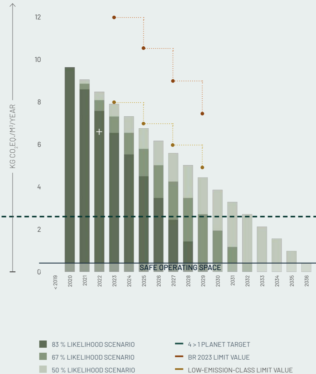
Figure ENF04.6: Reduction Roadmap The case study in relation to the Reduction Roadmap, limit values, the 4 to 1 planet goal of 2.5 kg CO 2 eq./m 2 /year, and the 'safe operating space'.
