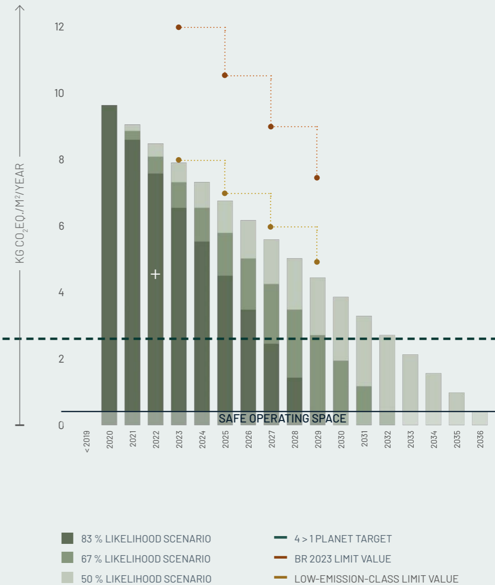
Figure R05.6: Reduction Roadmap The case study in relation to the Reduction Roadmap, limit values, the 4 to 1 planet goal of 2.5 kg CO 2 eq./m 2 /year, and the 'safe operating space'.
