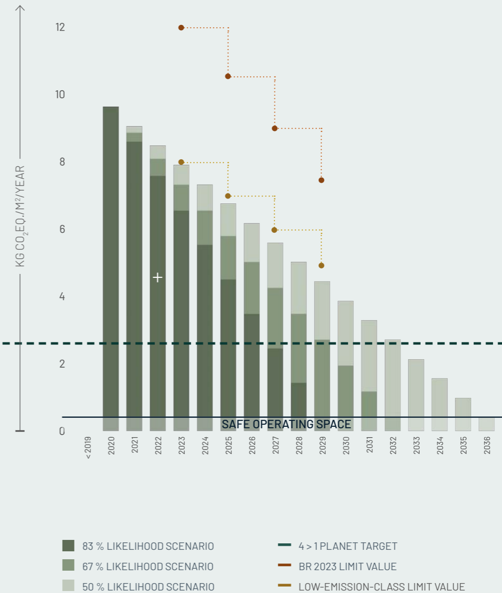
Figure R04.6: Reduction Roadmap The case study in relation to the Reduction Roadmap, limit values, the 4 to 1 planet goal of 2.5 kg CO 2 eq./m 2 /year, and the 'safe operating space'.
