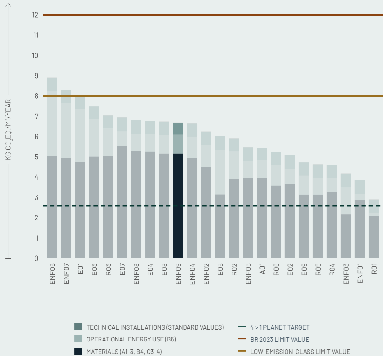
Figure ENF09.5: Housing case studies The vertical axis shows the emission of CO 2 eq./m 2 /year. The horizontal axis shows the 24 best practice cases.
