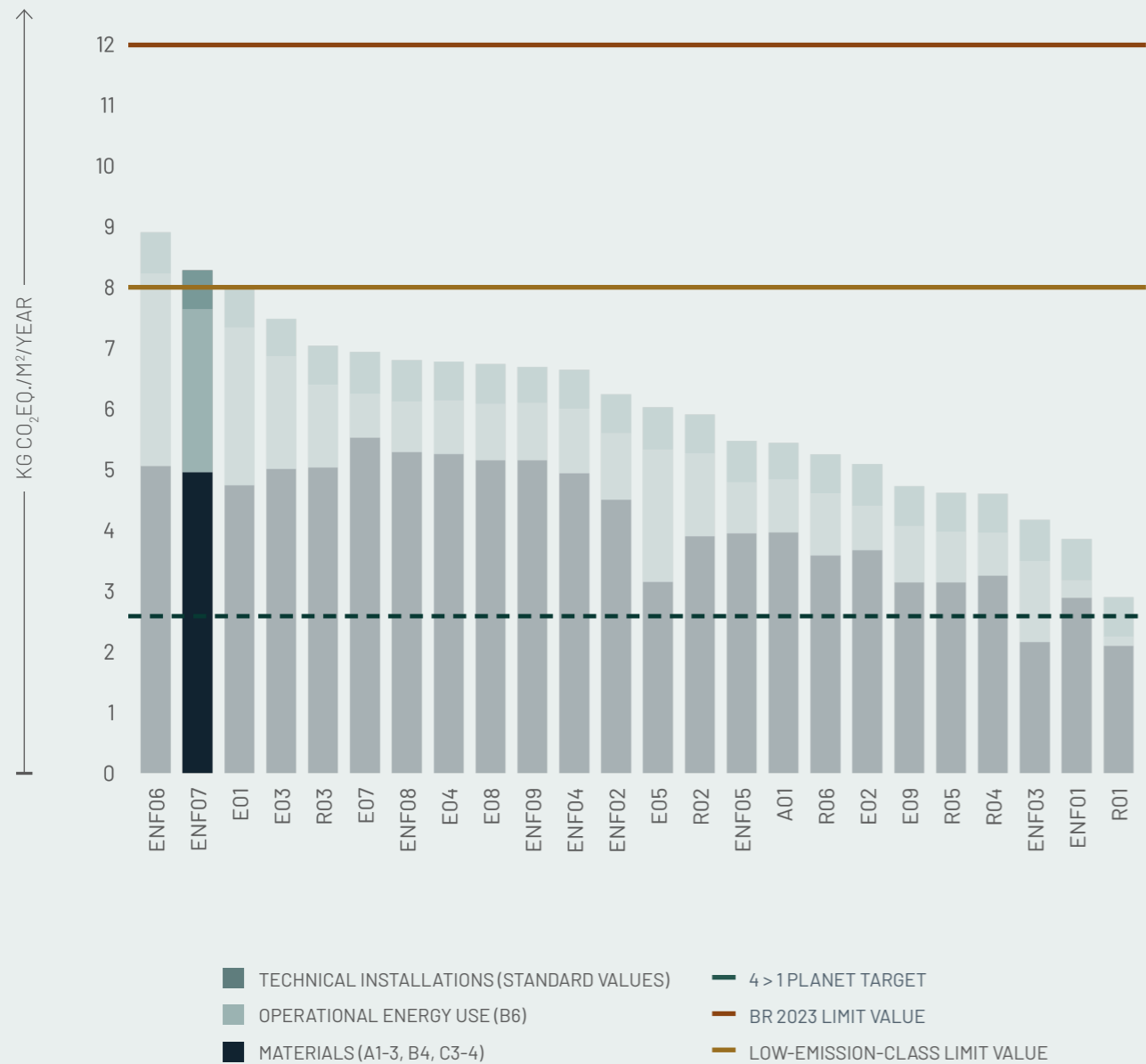
Figure ENF07.5: Housing case studies The vertical axis shows the emission of CO 2 eq./m 2 /year. The horizontal axis shows the 24 best practice cases.
