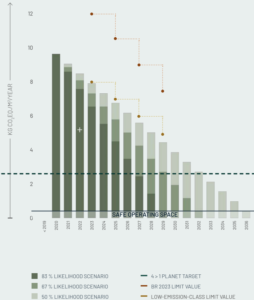
Figure R06.6: Reduction Roadmap The case study in relation to the Reduction Roadmap, limit values, the 4 to 1 planet goal of 2.5 kg CO 2 eq./m 2 /year, and the 'safe operating space'.
