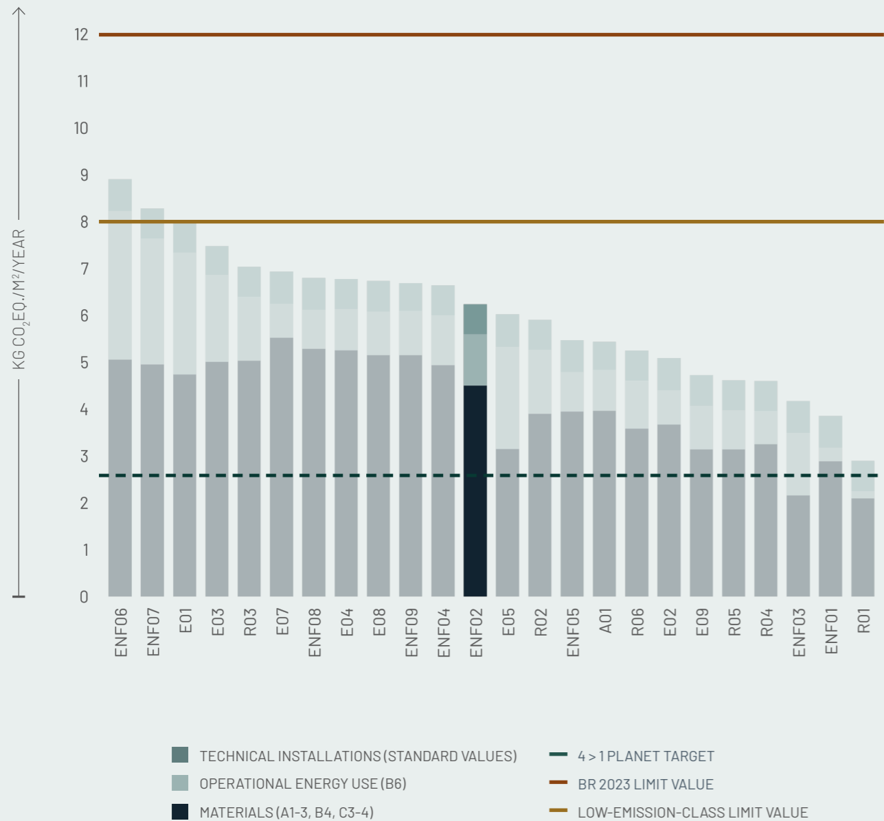
Figure ENF02.5: Housing case studies The vertical axis shows the emission of CO 2 eq./m 2 /year. The horizontal axis shows the 24 best practice cases.
