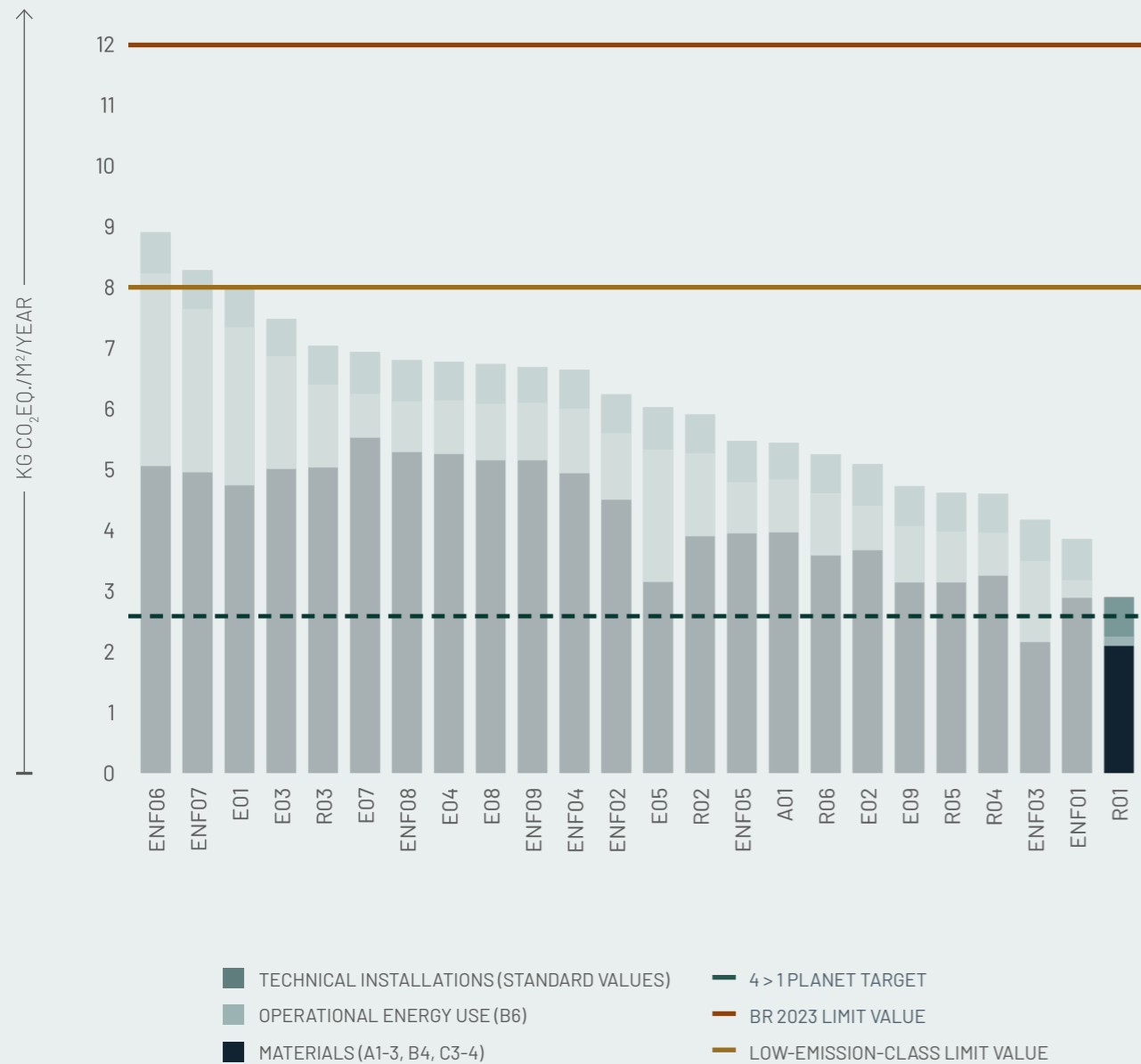
Figure R01.5: Housing case studies The vertical axis shows the emission of CO 2 eq./m 2 /year. The horizontal axis shows the 24 best practice cases.
