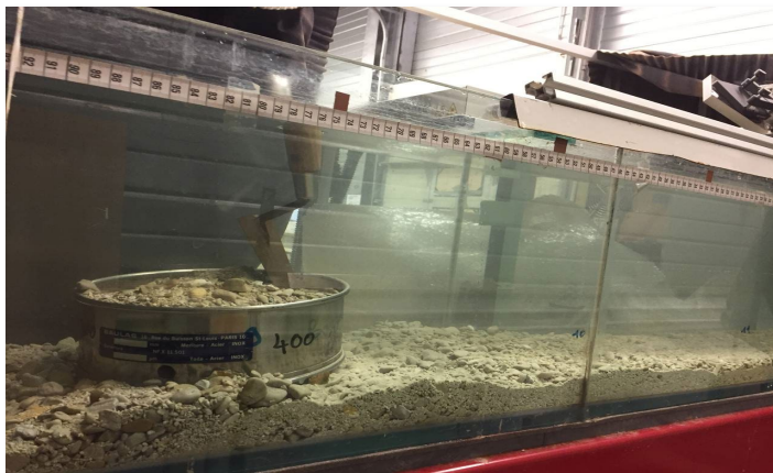
Fig 3-4. Rectangular glass flume
