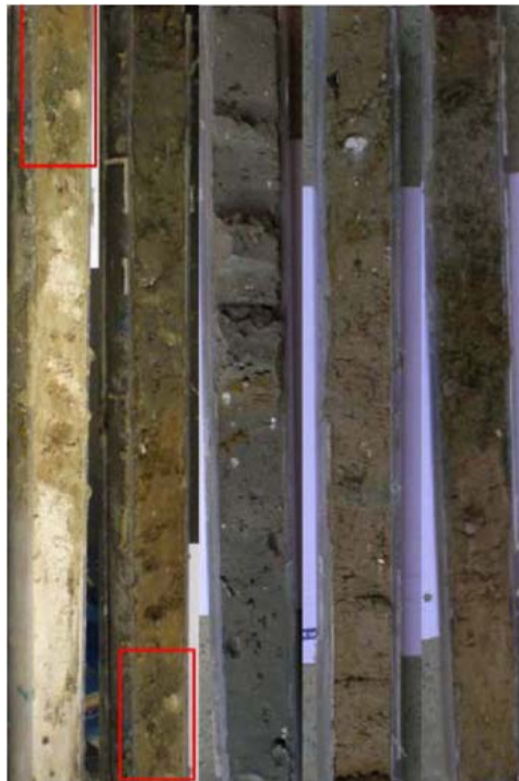
Figure 16. Examples of drill cores taken at the study site. The cores contain limestone (to the left) and various clay till materials. Red squares denote a contaminated sandy lens (Paper II).
