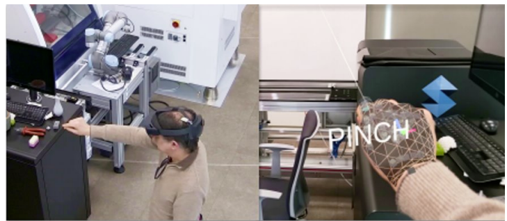
Figure 1: Left: dictionary of the gesture recognized by our Hololens 2 app. Right: the gesture recognition can be used to interact effectively with machines in an augmented workplace demo.
