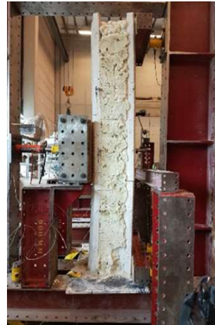
Fig. 6.18 Vertical flexural test [12]
