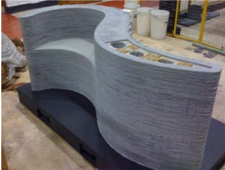
Fig. 6.9 Digital manufacturing of a free-shaped wall-like concrete bench [3]
