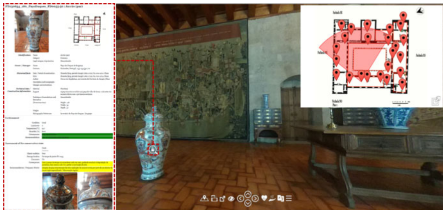
Figure 7. Virtual tour enriched with asset hotspots, linked to condition survey report.
