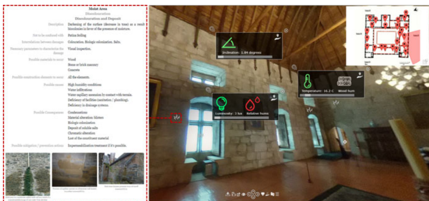
Figure 8. Virtual tour enriched with sensors and damage hotspots, linked to recent acquisition and damage report, respectively.
