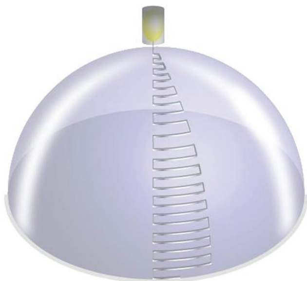
Figure 29. Drawing depicting the precise deposition of ink on a 3D construct through 5–6 DOF dispensing systems.
