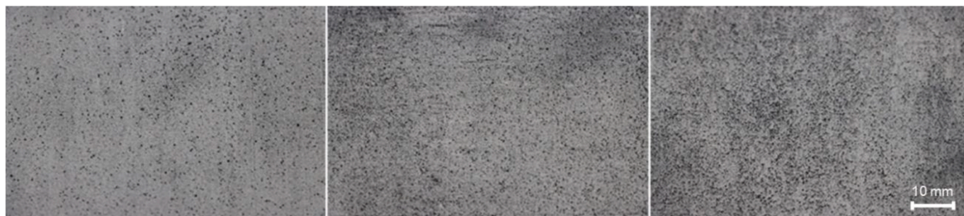
Fig. 1. Details of the top surface of test specimens produced by SLS with PA12 incorporating 0.50 wt% (left), 1.75 wt% (top) and 3.00 wt% (right) of MWCNT.
