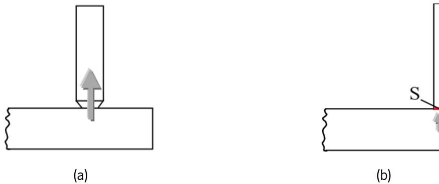
Figure 58: Air Venting (a) considered in the die; (b) considered only at the interface cavity/vent.
