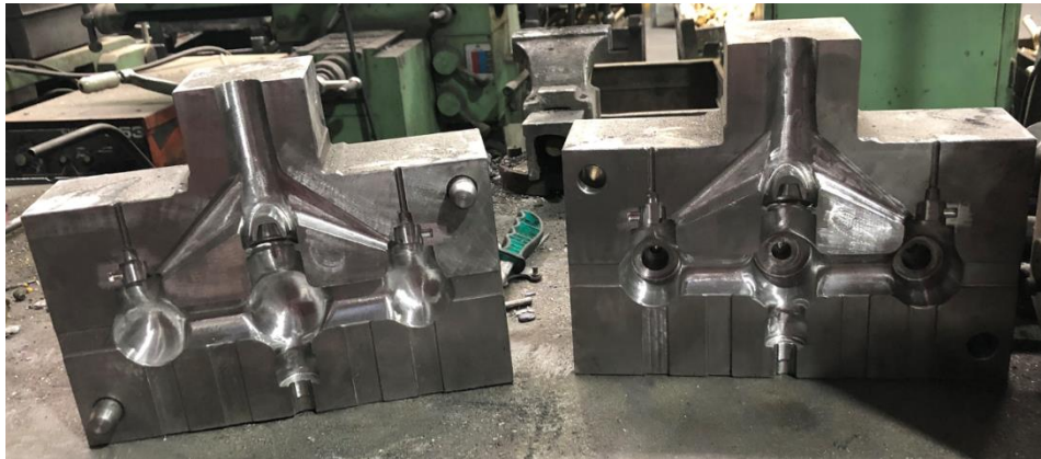
Figure 96: Final dies used for the production of the bathtub mixer.
