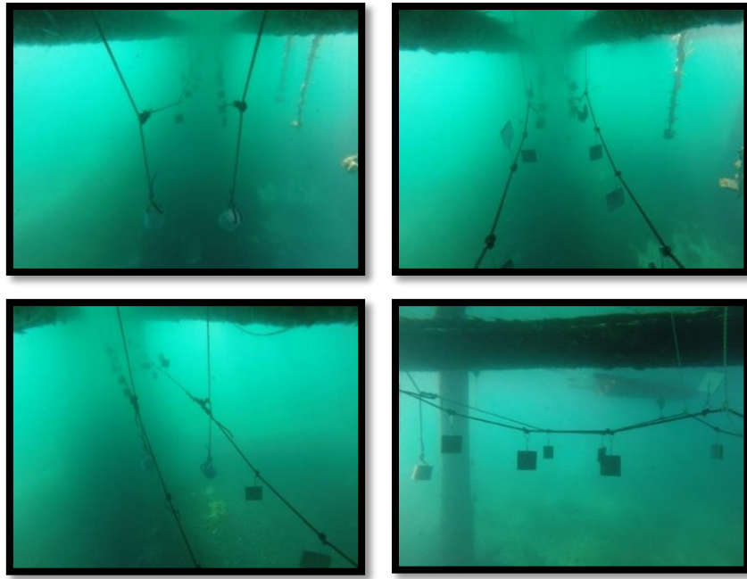
Figure S.4.1. Sampling set-up: substrates suspended horizontally and deployed in December 2016 at Toralla Island (NW Iberian Peninsula).
