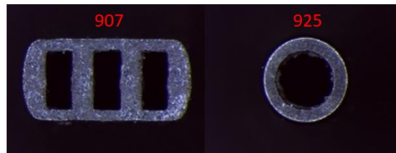
Fig. 5. Microscopic photography of nozzles 907 and 925.
