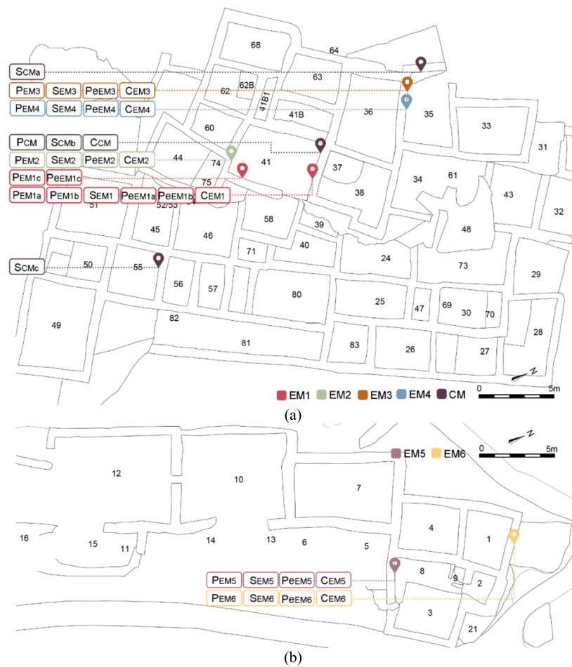
Fig. 10. Room numbering, location of tests and selected mortars: (a) South Unit, (b) North Unit.
