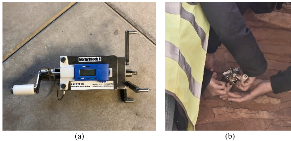
Fig. 6. Scratch test: (a) equipment; (b) in operation.
