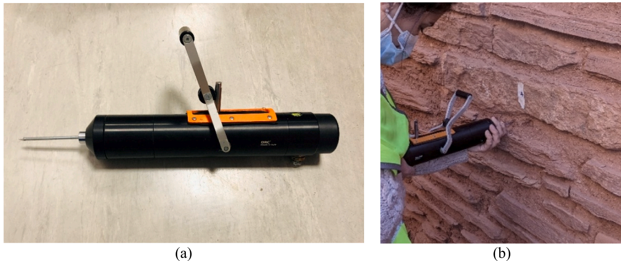
Fig. 1. Penetrometer test: (a) equipment; (b) in operation.
