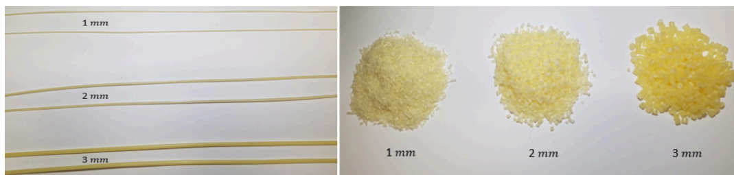
Figure 2 – Filaments and pellets of MDPE/ADCA masterbatch.
