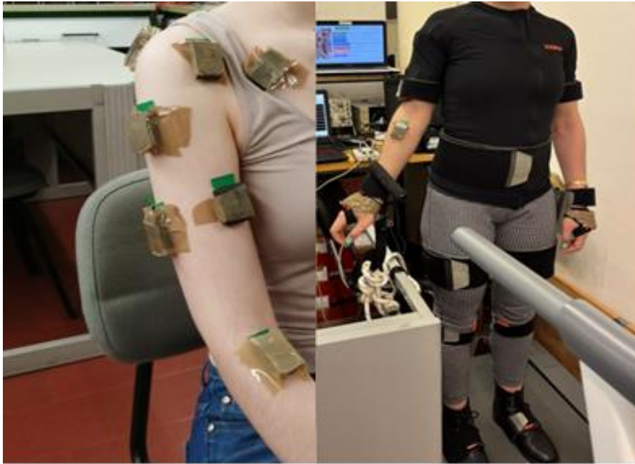
Figure 21 - Placement of EMG sensors (left) and Xsens suit with IMUs sensors (right).
