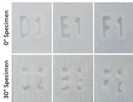
Figure 4 Resolution of fine details of SLS specimens at 0° and 30°
