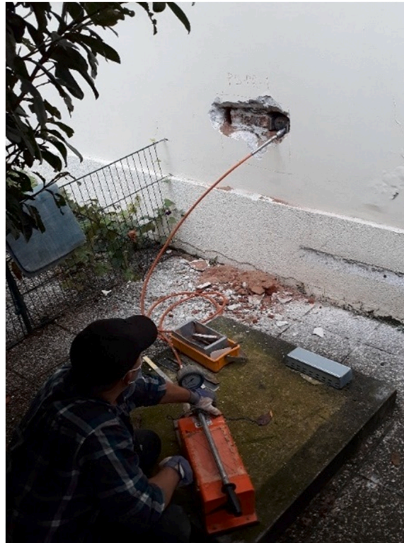
Fig. 8. Shear strength test of masonry [12].
