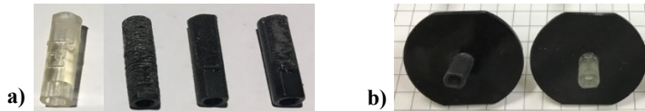
FIGURE 3. Prototypes of the 1003 nozzle: a) pipettes in the various materials; b) examples of the nozzles 1003 assembled.
