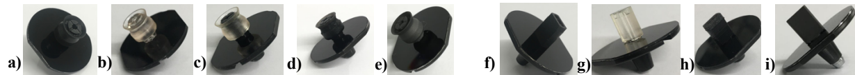
FIGURE 4. Prototypes of the nozzles 1005 and 2442: a) original 1005; b) Flexible 80A 1005; c) VeroBlack and Flexible 80A 1005; d) Agilus30 and VeroBlack 1005; e) appearance of nozzles 1005 with coating; f) Original 2442; g) Flexible 80A 2442; h) VeroBlack and Agilus30 2442; i) appearance of nozzles 2442 with coating.
