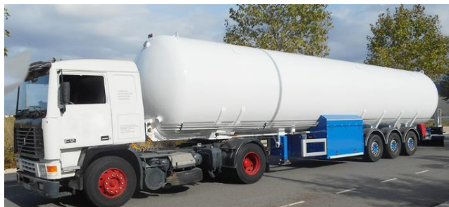
Figure 21 – Example of a truck trailer coupled with liquid hydrogen storage tank (Furui CIT, 2022).
