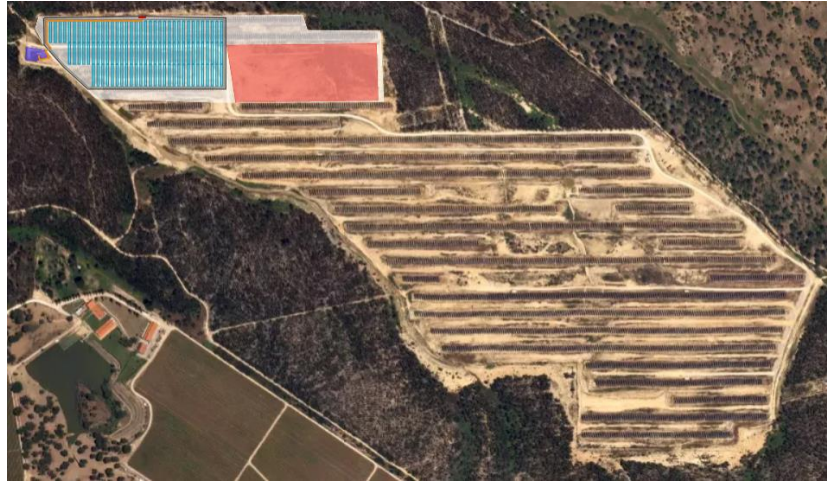
Figure 54 – Representation of the real PV power plant and the projected power plant. The blue rectangle represents the projected PV panels, while the black ones represent the actual PV panels.
