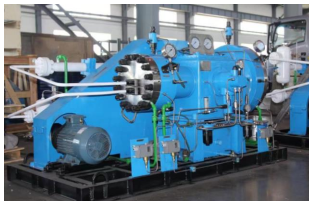
Figure 57 - Representation of the chosen hydrogen diaphragm compressor option from the Minnuo Group.
