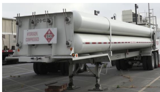
Figure 19 – Example of a truck trailer coupled with hydrogen gas storage bundled tubes (AIChE Academy, 2020).
