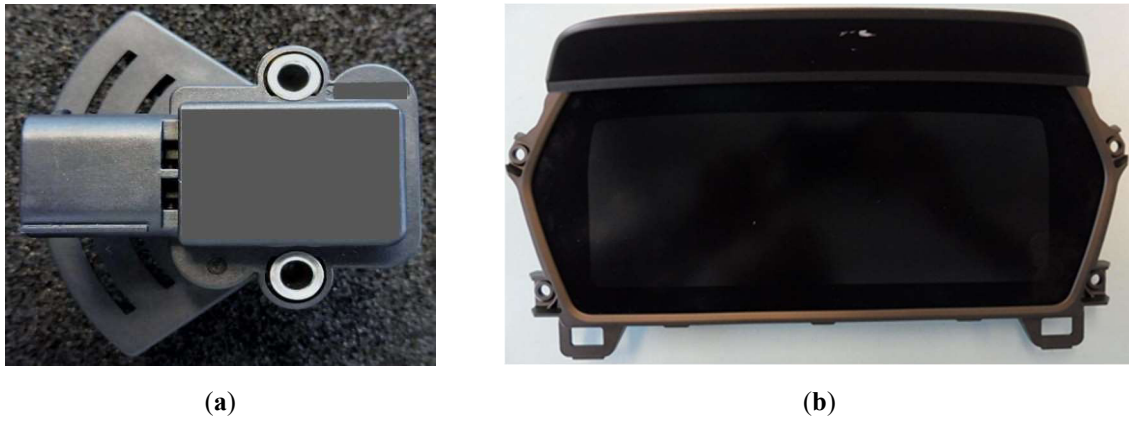
Figure 8 - (a) Chassis Sensor; (b) Instrument Cluster
