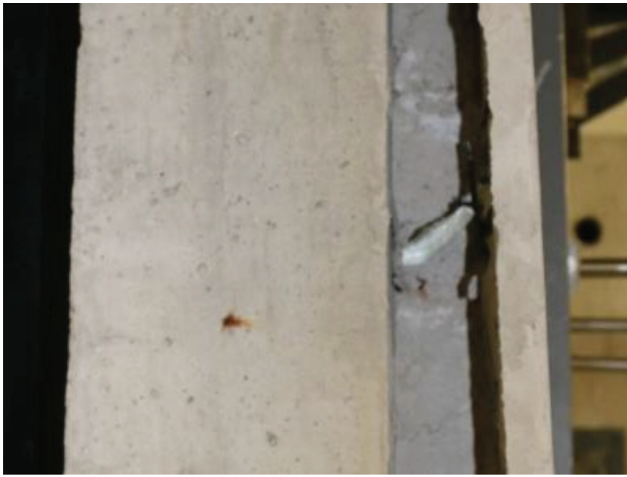
Figure 16. Detachment of the connectors from RC frame.
