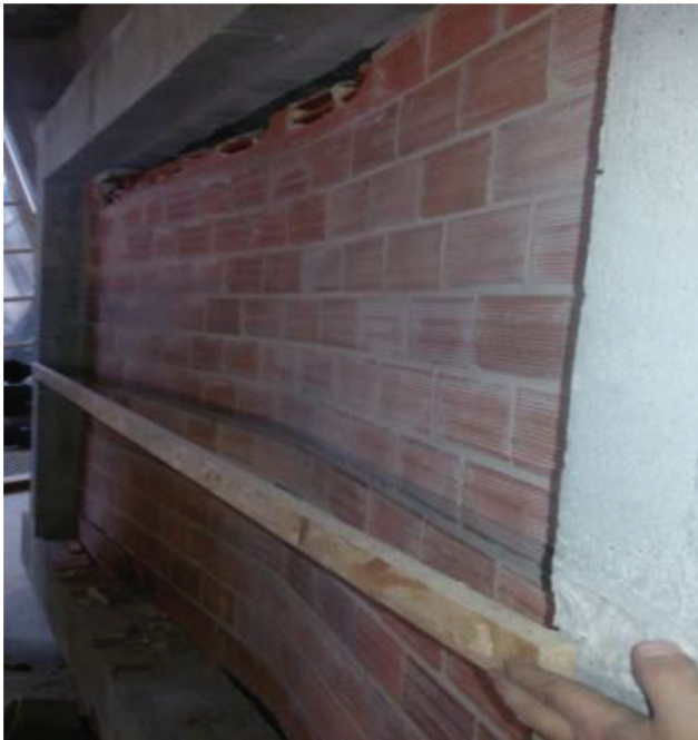
Figure 12. Final deformation of the infill.
