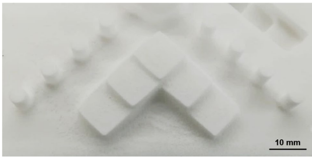
Fig. 5 Surface of an artifact test produced by SLS with 0.358 \text{ J/mm}^3 (after sand blasting)
