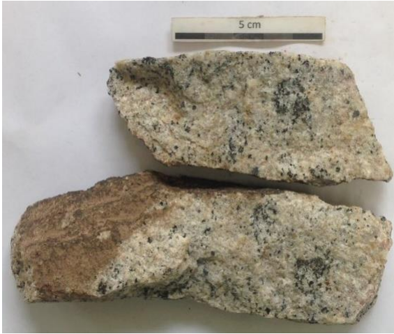
Figure 3. Pegmatite sample, classified as Quartz alkali feldspar in the QAP Diagram, with K-feldspar grain size between < 1\text{ mm} and 3\text{ mm} , biotite grains size between <1\text{ mm} to 3\text{ mm} , and quartz grain size between <1\text{ mm} and 2\text{ mm} , collected at the Jatobá Mine.
