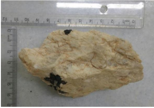
Figure 4. Pegmatite rock sample, classified as a Tonalite in the QAP Diagram [12], with plagioclase grain size between <1 mm and 1.5 cm, quartz grains size between <1 mm to 1.3 cm, and black tourmaline grain size between <1 mm and 1.5 cm, collected at Duas Cores Mine.
