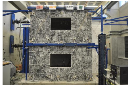
Figure 5. Building façade that DIC was applied
