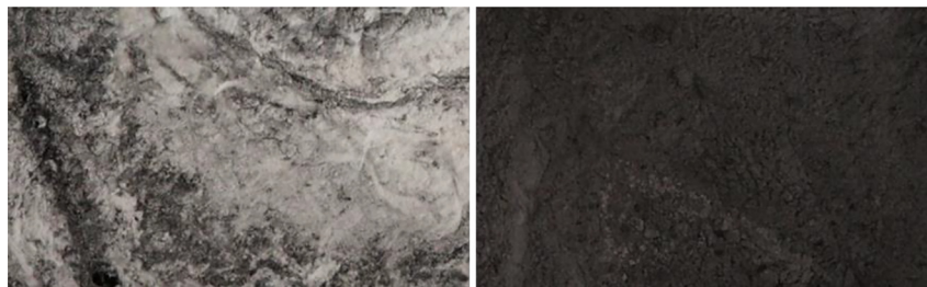
Figure 3 Mechanical mixing of PA12-GNP materials in initial (left) and final (right) stages
