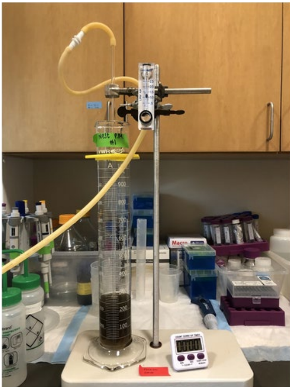
FIGURE 1 Apparatus to measure foaming potential of activated sludge. The apparatus was connected to controlled air flow in a fume hood. The diffuser was submerged in the activated sludge sample. Foaming potential was measured by observing the foam volume in the graduated cylinder.
