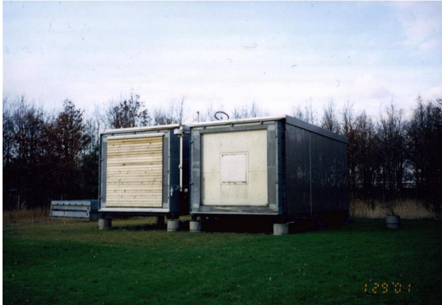
Figure 3 Photo of two PASSYS test cells at the Technical University of Denmark, one of which is used for the validation of BSim2000 's moisture model.
