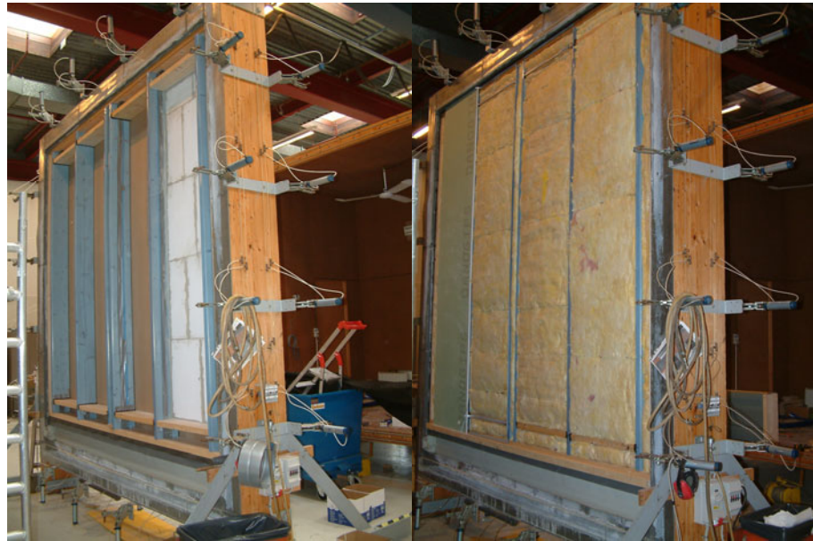
Figure 2. The test rig with the four elements seen from the outdoor side before (left) and after (right) mounting the thermal insulation. Element 4 at right.
