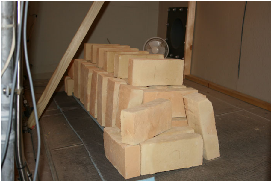
Figure A11. Placement of bricks at the outdoor side to increase the thermal mass for stabilising the temperature. Fans are added in order to ensure that the bricks are activated as thermal mass.
