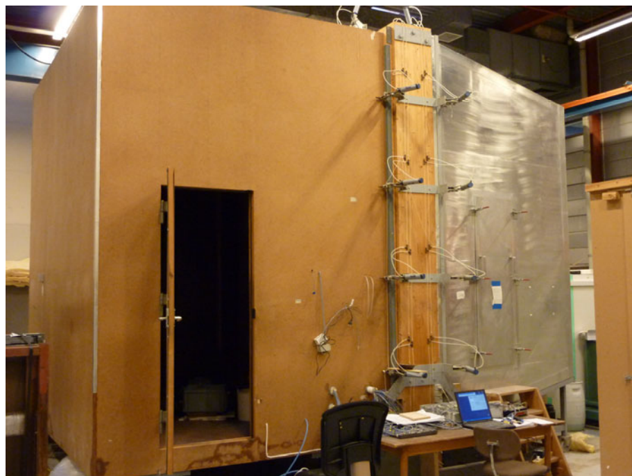
Figure A8. Climate simulator at SBI. Indoor side at left, outdoor side at right.
