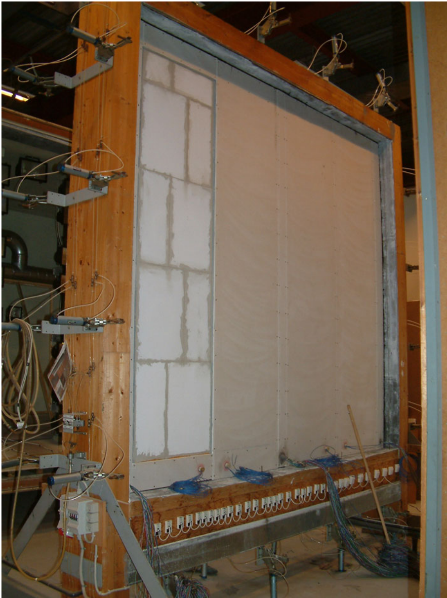
Figure 3. The test rig with the four test elements seen from the indoor side with gypsum board as inner cladding at three of the four elements. The wires coming from the sensors inside the elements are seen at the bottom of each element.
