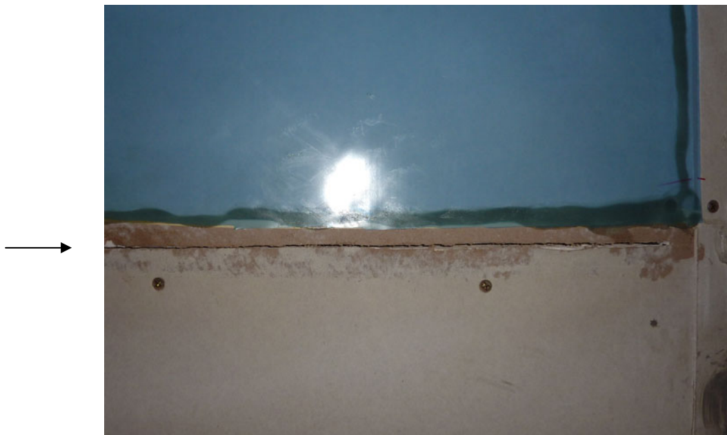
Figure A13. Element 3 with a slit (see arrow) below the vapour barrier.
