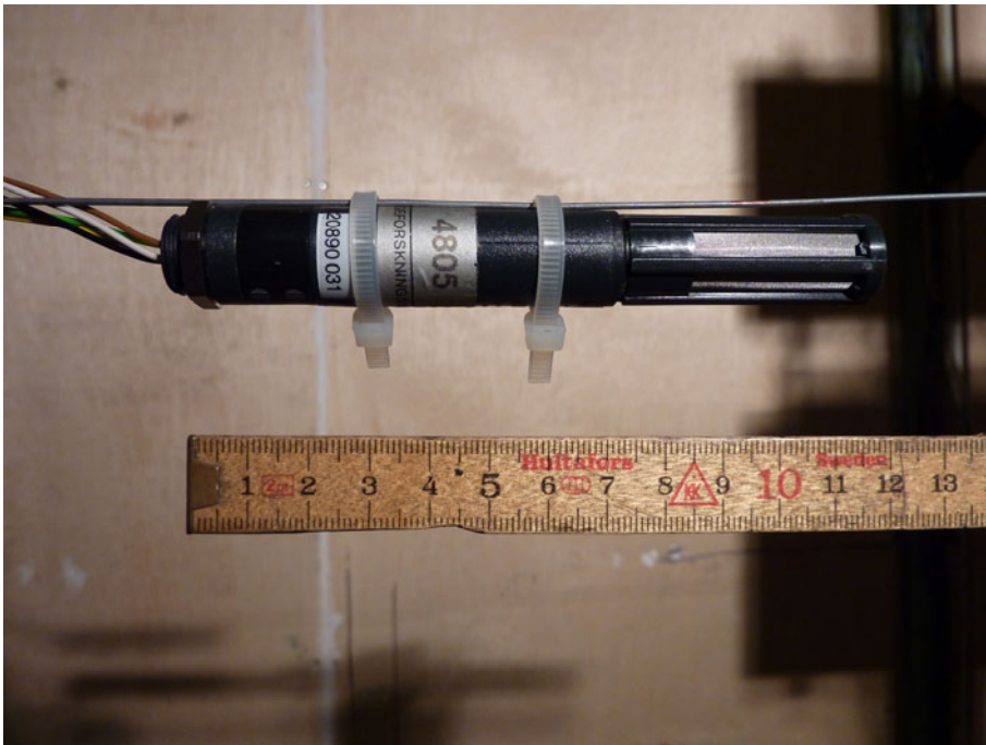
Figure A18. RH sensor (Rotronic). Specifications: see Table A1.
