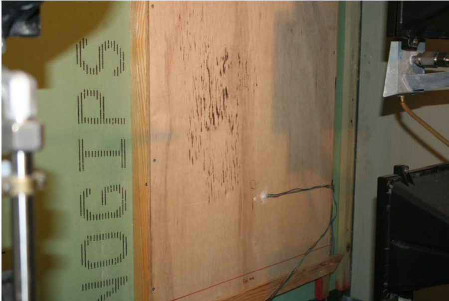
Figure A14. Element 4 seen from the outdoor side after mounting the cladding. The sensors are fixed at the back (indoor) side of the cladding while the wires are led on the outdoor side in order to disturb the conditions in the cavity as little as possible.
