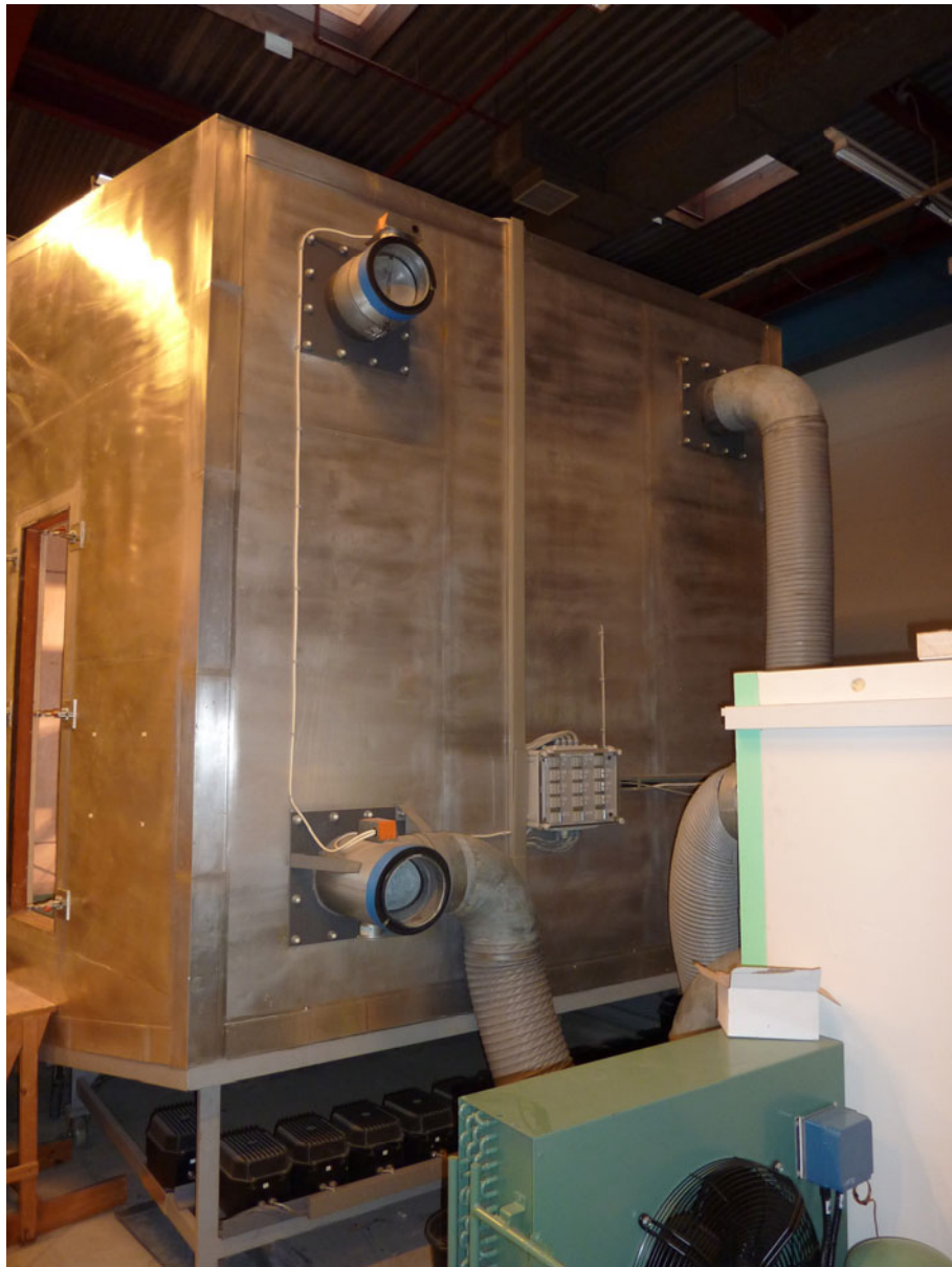
Figure A20. Climate simulator with inlet (top) and outlet (bottom) at the outdoor climate chamber for air from and to the cooling machine.
