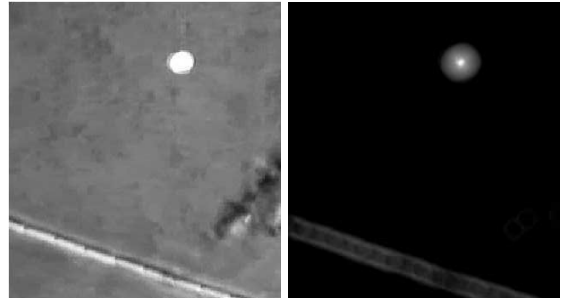
Figure 5: Left: Input to the Hough transform; the slung load can be seen in the upper half of the picture. Right: Output of the Hough transform from which the load can be easily located by a peak detector.
