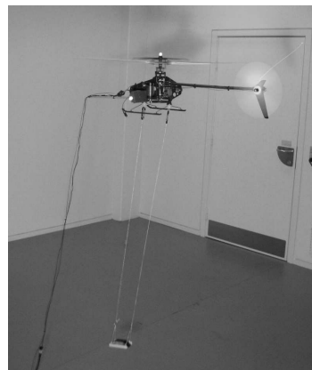
Figure 11: The Aalborg University Corona flying indoor with slung load.
