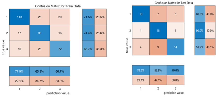
Figure 10. Confusion matrix for ELM using HSI (1), GLCM (2) and HSI fused with GLCM (3)
