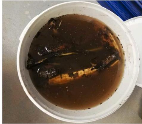
Fig. 11. Solution of *beini* used for the earth-based mortars (photograph by the authors).
