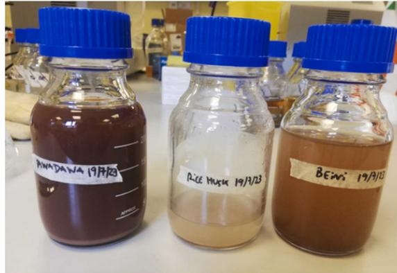
**Fig. 12.** Filtered solutions of macerated *dawadawa*, *beini* and rice husk (photograph by the authors).
