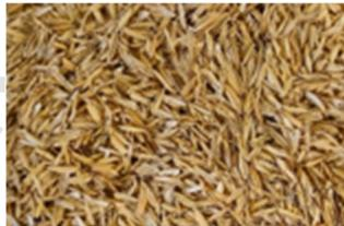
Fig. 8. Rice husk was used for mortar preparation (photograph by the authors).
