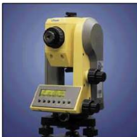
Figure 4. Electronic total station Trimble 3300 DR. Source: Trimble (2004)
