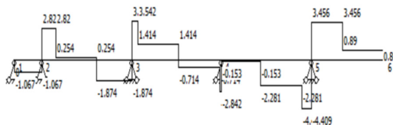
Figure 16. Calculation diagram for shear resistance of left upper flipped side template.
