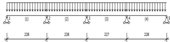
Figure 9. Calculation diagram for left upper flipped side template.
