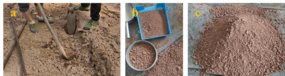
Fig. 1. Some of the processes of the experiment (a: Collection of experimental soil samples, b: Sieving of soil samples, c: Mixing of soil samples)
