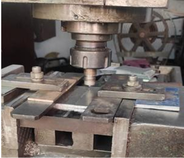
Figure:2 Plates joint process in FSW
