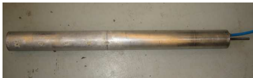
Figure 6: Picture of the test pile with an outer diameter of 80 mm. The cords are lead out through the blue cable.
