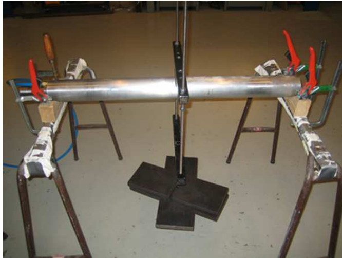
Figure 9: Test setup for calibration of pile bending stiffness, E_p I_p , and validation of strain gauges.
