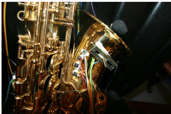
Figure 1: Closeup of the fader and pushbuttons on the psychoPhone
