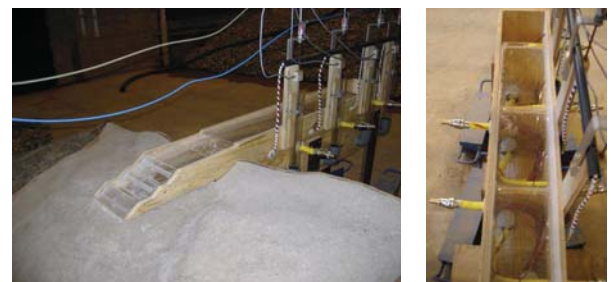
Figure 3. Details of the model in scale 1:60: on the left a top view of the rear tank containers equipped with pumps.
