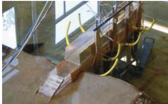
Figure 9: Model for 3D overtopping tests.
