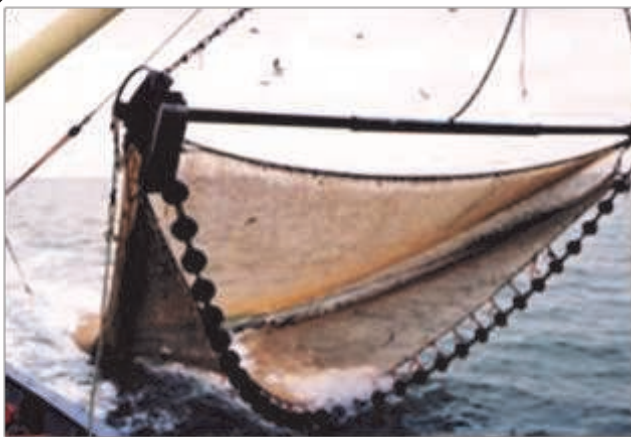
The Nephrops fishery utilises mainly demersal trawls with a mesh size of 70-99mm. Other mesh sizes are also used and different rules apply to different net constructions in different Economic zones.
