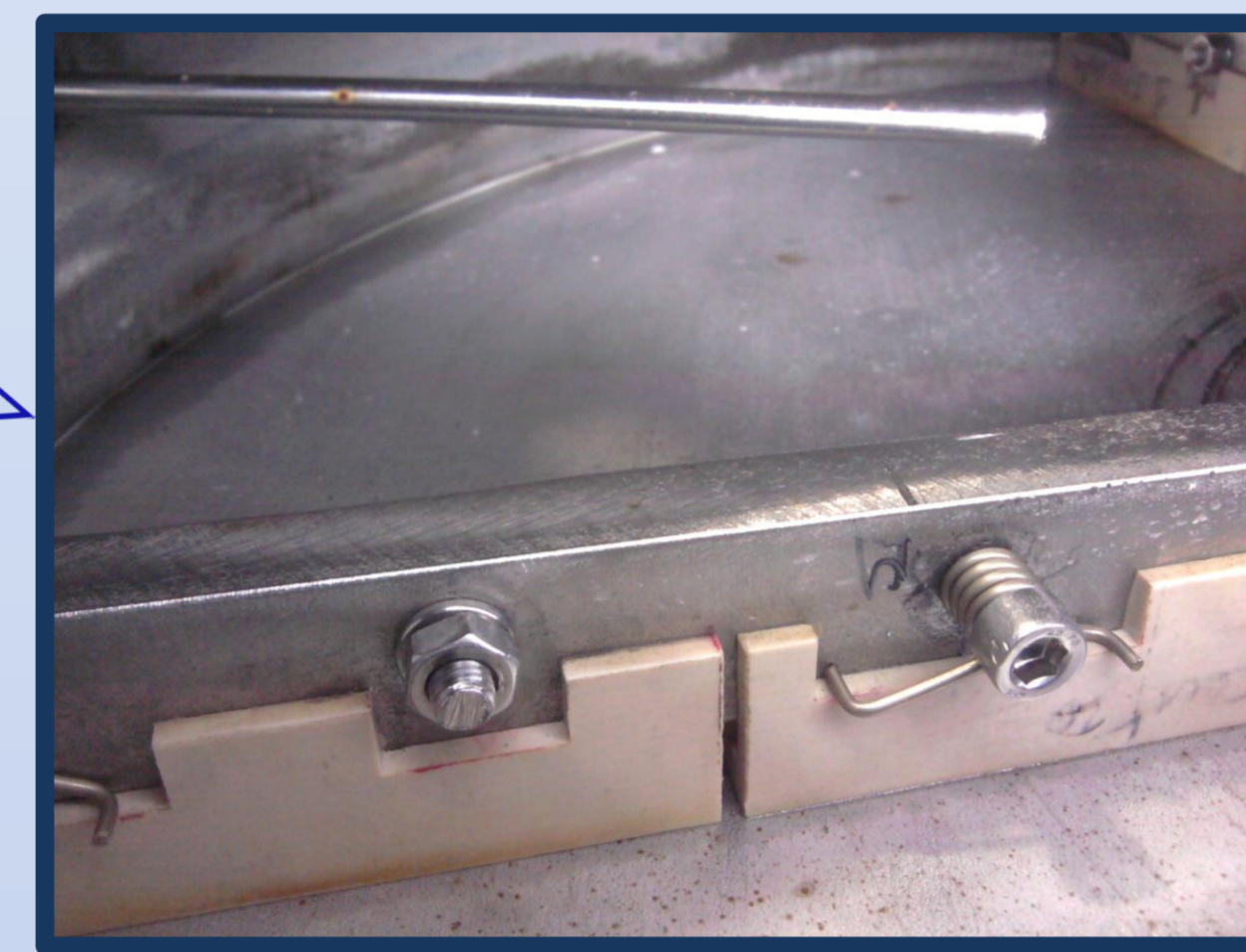
Scraper blades with the springs of the adaptive contact system
