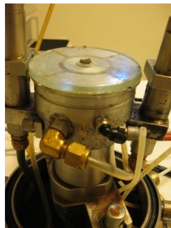
Figure 5.7 Pore pressure transducer built into pressure head.
