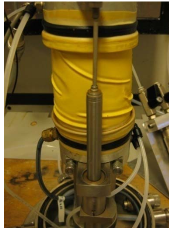
Figure 5.4 Displacement transducer installed in cell.
