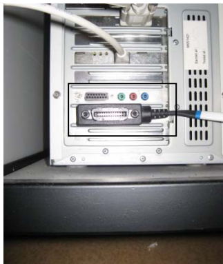
Figure 6.1 Cable between MGCplus and computer connected to computer.
