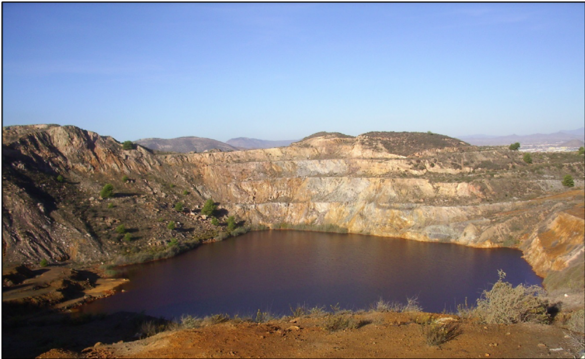
Figure 2.11. The open-pit mine “Brunita” and the acid lake formed by the excavation below groundwater level.
