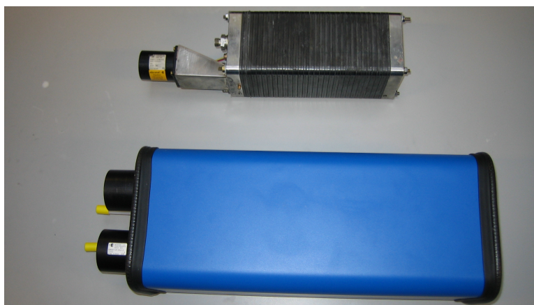
Figure 4.1: Top: 30 cell HTPEM fuel cell stack, initial prototype stack. Bottom: 65 cell HTPEM fuel cell stack, commercial stack from Serenergy.
