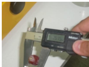
Picture 3. Measurement of berries geometrical characteristics with digital calliper
