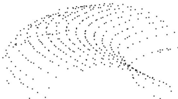
Fig. 5. Clouth of points obtained with Photomodeler Scanner
