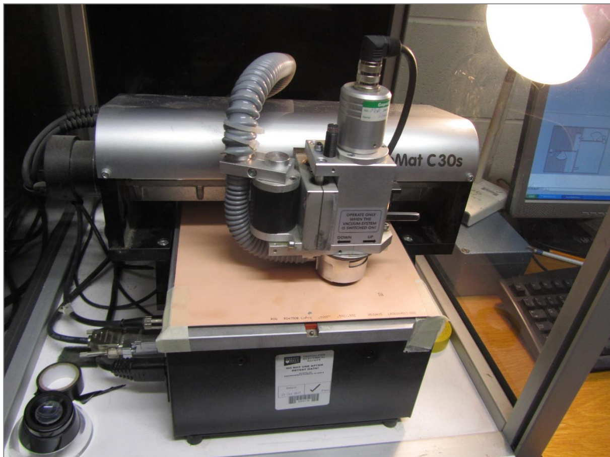
Figure 4.7 – Starting the milling process with ProtoMat C30s.
