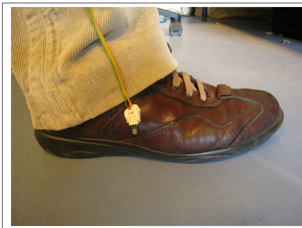
Figure 1: The contact microphone attached to the shoe.
