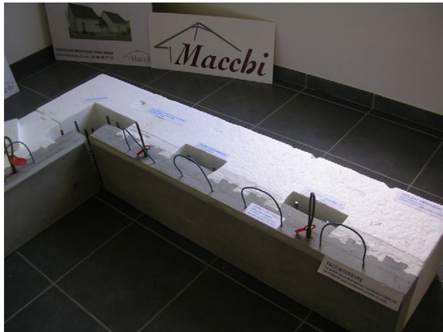
Figure 17: Electric networks integrated in the prefabricated walls. (Foto: Frédéric Bougrain).
