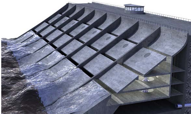
Figure 1 - Scheme of Seawave Slot-Cone Generator
