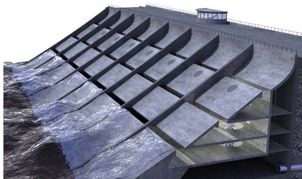
Figure 1 - Scheme of Seawave Slot-Cone Generator
